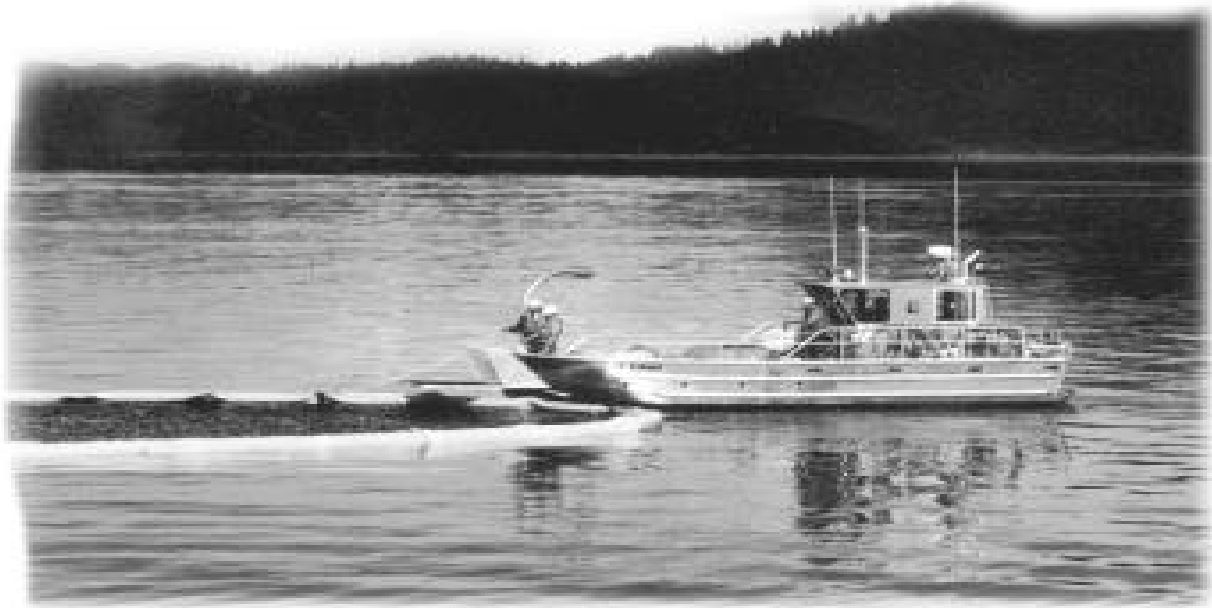
High speed response vessel executing a "U configuration" boom response near Juneau in May, 1994. Alaska Department of Environmental Conservation.
